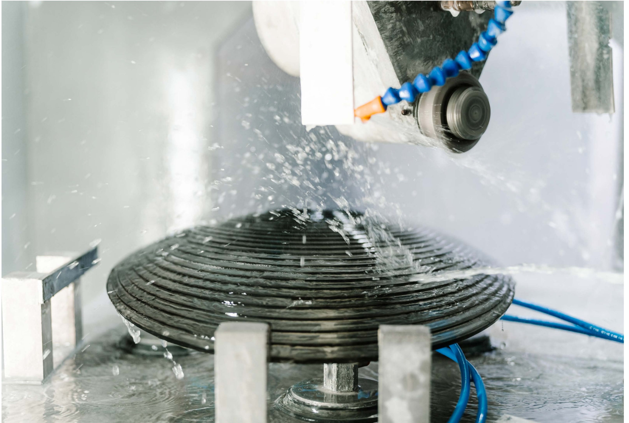
Each glass shell is meticulously cutted by in-house developed machines.
