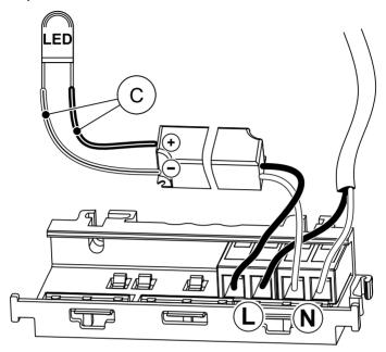
Carry out this step in reverse to fit the new LED module. Plug in the light again.
