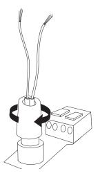
Lead the cables through the holes at the canopy. Each cable is marked with a number from 1 to 8. Arrange the cables by numbers.
