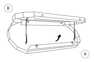
Lift up the ceiling plate (A) until it is fixed to the ceiling base (B) . A "click" sound will indicate correct mounting.
