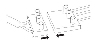
Disconnect the plug (1) and lead the power cable into the empty plug part (2).
