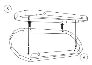
Attach the 2 wire the from celing base (B) to the hooks in celinge plate (A)
