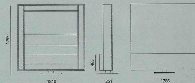
Metal basement with satin finish. Structure in black tubular. Glass door on a black anodized aluminium framework. Mirror back on a black anodized aluminium framework.
