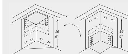
A special metal support allows to place the slats in different positions from 2 cm - 3/4" to 18 cm - 7" from the edge of the bed base.
