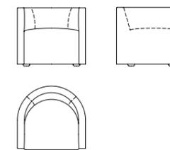
For weaved or striped fabrics, the inner covering of the backrest is done with two seams.
