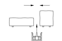
Hooks for assembly elements with feet with spacers.
