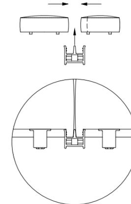
Hooks for assembly elements with feet with spacers.
