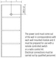
The power cord must come out of the wall in correspondence with each wall mounted module and it must be prepared for use with a remote controlled switch or a radio control kit. Electrical connections must be
