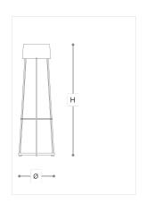
Reading lamp with blown glass diffuser with shaded titanium finish. Metal structure with iron grey finish and shelves in "fumè" glass. Double LED source with double switching system.
