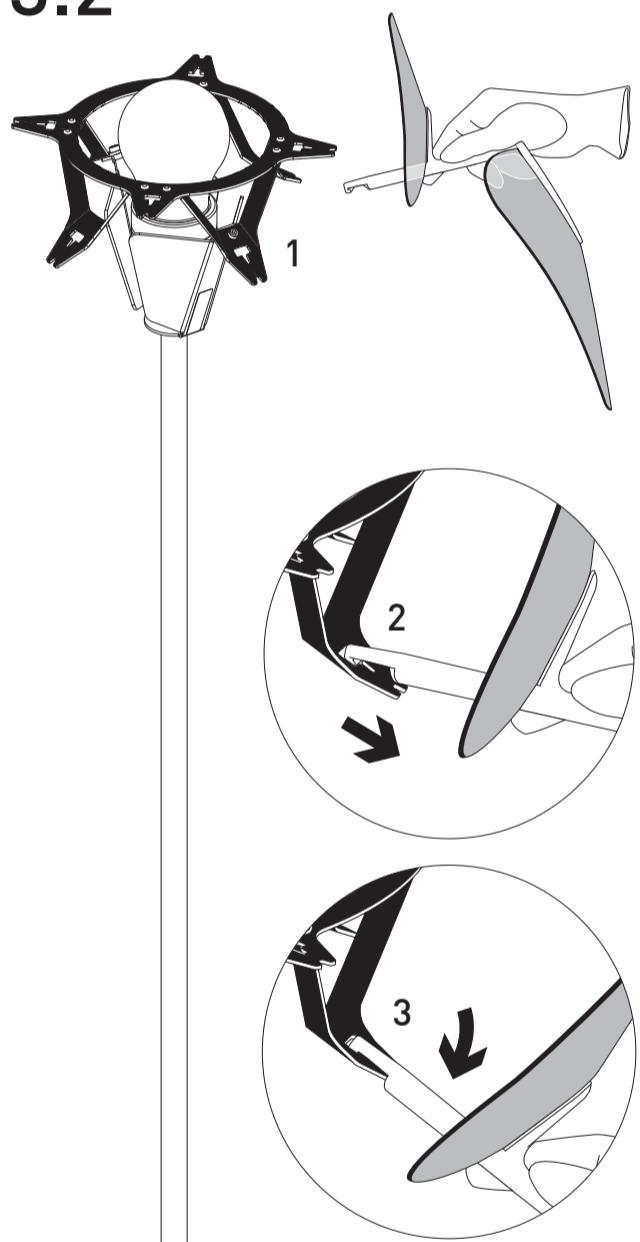
3.2 In order mate each arm, insert it from above as shown in fig. 1, pull it to the outside (fig. 2) letting it simply lower until the stop (fig. 3).
