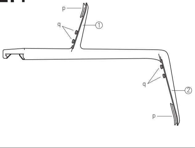
2.1 Every arm has a short bracket (above) [1] for the small lens and a longer one (lower) [2] for the big lens. The two brackets have a guide (p) to engage the lenses and two pegs (q) for their fastening.
