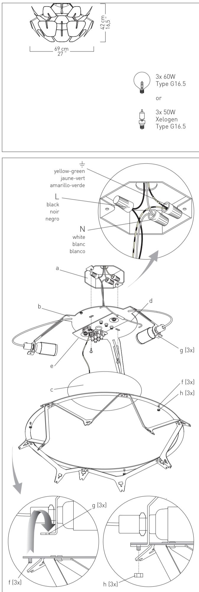
Carry out the electrical connections to the junction box [a] by respecting the polarities indicated in the figure.
