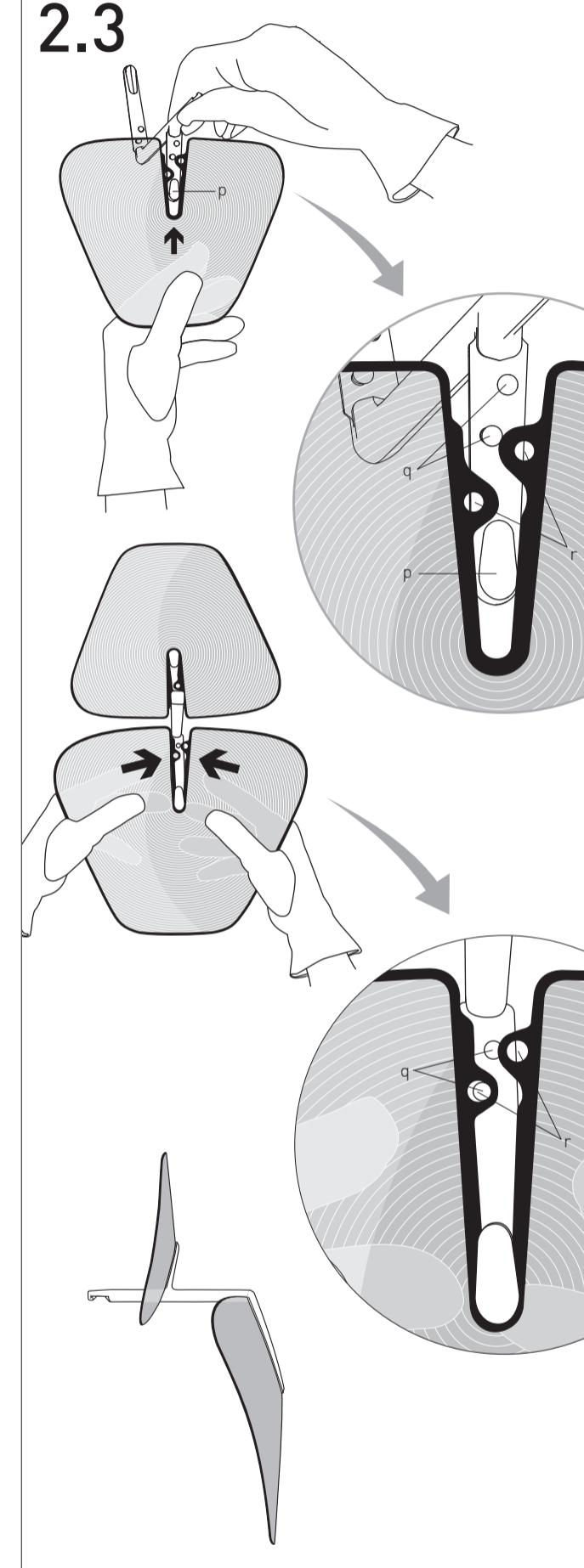
2.3 To mount the lens on the arm slide it onto the guide (p) of the bracket and then engage the two holes (r) onto the pegs (q). First engage the inner hole of the lens, then the outer one, giving the lens the necessary bend.
