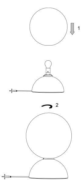
Screw the bulb in the socket clockwise. Use E27 bulb with the following specifications: max. 20W, 220–240V. The manufacturer shall not be held responsible for improper function when other light source is used.
