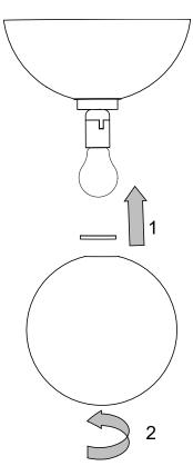
Carry out this step in reverse to fit the new bulb.
