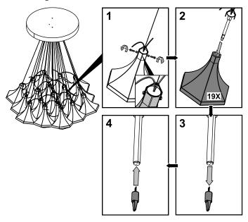
Carry out this step in reverse to fit the new bulb.
