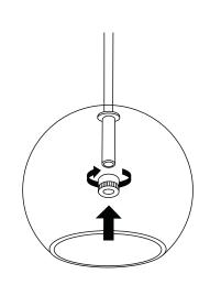
Remove the screw from the metal tubes by hand. Mount the glass-ball. Replace the screw carefully. **NB.** Tighten gently!
