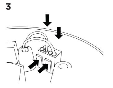
Lead the ends of the wires in through the plugs. Place one wire-end in one of the two holes to the right side, place the other wire-end in one of the two holes to the left side. (See drawing)
