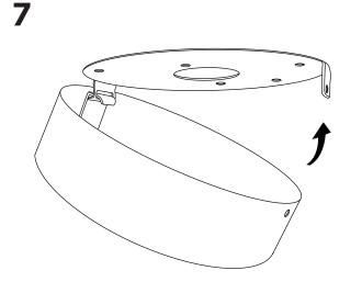
Rotate the canopy to horiziontal position.
