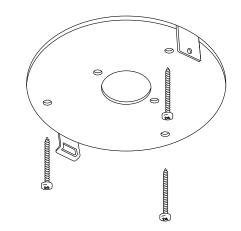
Mount the top plate of the canopy at the ceiling and fix with screws.
