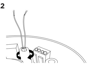
Tighten the wire by turning the white screw clockwise.
