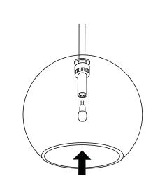
Place the 10 watt halogen bulb in the socket. **NB.** The bulb should not be in directly contact with skin at any time !
