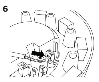
Lead the 230 volt wire into the plugs in centre of the canopy.
